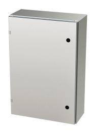
Saginaw Enviroline series enclosure, NEMA 3R/4/4X/12/13,  $30 \times 20 \times 8$  in (HxWxD), wall mount, 316L stainless steel, #4 brush finish, single-door, 1/4-turn semi-flush latch.
