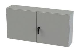
Saginaw enclosure, NEMA 3R/12/13, 30 x 60 x 12in (HxWxD), wall mount, carbon steel, ANSI 61 gray, powder coat finish, doubledoor, 3-point keylocking/padlocking combo handle.
