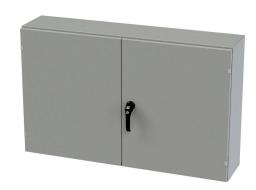
Saginaw enclosure, NEMA 3R/12/13, 30 x 48 x 10in (HxWxD), wall mount, carbon steel, ANSI 61 gray, powder coat finish, doubledoor, 3-point keylocking/padlocking combo handle.
