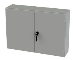
Saginaw enclosure, NEMA 3R/12/13, 30 x 42 x 10in (HxWxD), wall mount, carbon steel, ANSI 61 gray, powder coat finish, doubledoor, 3-point keylocking/padlocking combo handle.
