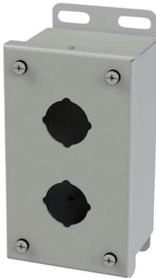
Saginaw pushbutton enclosure, 2 holes, 30mm, NEMA 4/12/13, 6 x 4 x 3in (HxWxD), wall mount, carbon steel, ANSI 61 gray, powder coat finish, screw cover.
