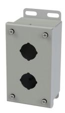
Saginaw pushbutton enclosure, 2 holes, 30mm, NEMA 4/12/13, 6 x 4 x 3in (HxWxD), wall mount, carbon steel, ANSI 61 gray, powder coat finish, screw cover.
