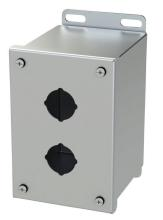
Saginaw pushbutton enclosure, 2 holes, 30mm, NEMA 4/4X/12/13, 6 x 4 x 5in (HxWxD), wall mount, 316L stainless steel, #4 brush finish, screw cover.
