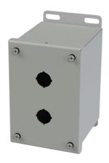
Saginaw pushbutton enclosure, 2 holes, 22mm, NEMA 4/12/13, 6 x 4 x 5in (HxWxD), wall mount, carbon steel, ANSI 61 gray, powder coat finish, screw cover.
