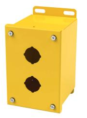
Saginaw pushbutton enclosure, 2 holes, 30mm, NEMA 4/12/13, 6 x 4 x 5in (HxWxD), wall mount, carbon steel, RAL 1018 yellow, powder coat finish, screw cover.
