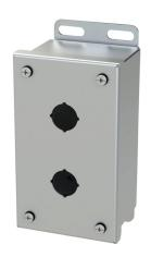
Saginaw pushbutton enclosure, 2 holes, 22mm, NEMA 4/4X/12/13, 6 x 4 x 3in (HxWxD), wall mount, 304 stainless steel, #4 brush finish, screw cover.
