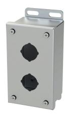
Saginaw pushbutton enclosure, 2 holes, 30mm, NEMA 4/4X/12/13, 6 x 4 x 3in (HxWxD), wall mount, 316L stainless steel, #4 brush finish, screw cover.
