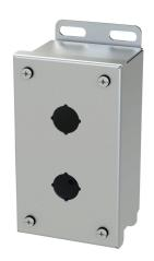
Saginaw pushbutton enclosure, 2 holes, 22mm, NEMA 4/4X/12/13, 6 x 4 x 3in (HxWxD), wall mount, 316L stainless steel, #4 brush finish, screw cover.
