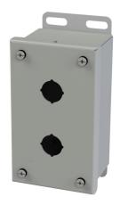
Saginaw pushbutton enclosure, 2 holes, 22mm, NEMA 4/12/13, 6 x 4 x 3in (HxWxD), wall mount, carbon steel, ANSI 61 gray, powder coat finish, screw cover.
