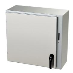
Saginaw Enviroline series disconnect enclosure, NEMA 3R/4/4X/12/13, right flange, 24 x 25 x 10in (HxWxD), wall mount, 304 stainless steel, #4 brush finish, single-door, 2-point padlocking handle, purchase subpanel separately.
