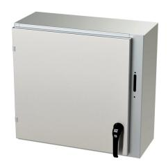
Saginaw Enviroline series disconnect enclosure, NEMA 3R/4/4X/12/13, right flange, 24 x 25 x 10in (HxWxD), wall mount, 316L stainless steel, #4 brush finish, single-door, 2-point padlocking handle, purchase subpanel separately.
