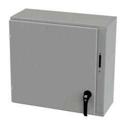
Saginaw Enviroline series disconnect enclosure, NEMA 3R/4/12/13, right flange, 24 x 25 x 10in (HxWxD), wall mount, carbon steel, ANSI 61 gray, powder coat finish, single-door, 2-point padlocking handle, purchase subpanel separately.
