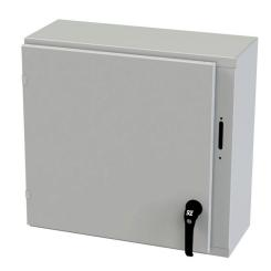
Saginaw Enviroline series disconnect enclosure, NEMA 3R/4/12/13, right flange, 24 x 25 x 10in (HxWxD), wall mount, carbon steel, RAL 7035 light gray, powder coat finish, single-door, 2-point padlocking handle, purchase subpanel separately.
