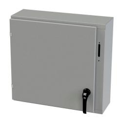
Saginaw Enviroline series disconnect enclosure, NEMA 3R/4/12/13, right flange, 24 x 25 x 8in (HxWxD), wall mount, carbon steel, ANSI 61 gray, powder coat finish, single-door, 2-point padlocking handle, purchase subpanel separately.
