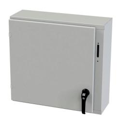
Saginaw Enviroline series disconnect enclosure, NEMA 3R/4/12/13, right flange, 24 x 25 x 8in (HxWxD), wall mount, carbon steel, RAL 7035 light gray, powder coat finish, single-door, 2-point padlocking handle, purchase subpanel separately.
