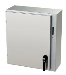
Saginaw Enviroline series disconnect enclosure, NEMA 3R/4/4X/12/13, right flange, 24 x 21 x 8in (HxWxD), wall mount, 304 stainless steel, #4 brush finish, single-door, 2-point padlocking handle, purchase subpanel separately.
