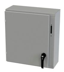
Saginaw Enviroline series disconnect enclosure, NEMA 3R/4/12/13, right flange, 24 x 21 x 8in (HxWxD), wall mount, carbon steel, ANSI 61 gray, powder coat finish, single-door, 2-point padlocking handle, purchase subpanel separately.
