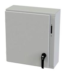
Saginaw Enviroline series disconnect enclosure, NEMA 3R/4/12/13, right flange, 24 x 21 x 8in (HxWxD), wall mount, carbon steel, RAL 7035 light gray, powder coat finish, single-door, 2-point padlocking handle, purchase subpanel separately.
