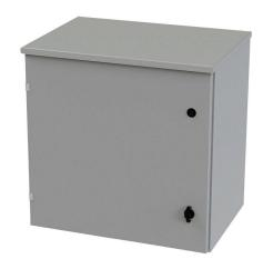
Saginaw enclosure, NEMA 3R, 24 x 24 x 16in (HxWxD), wall mount, carbon steel, ANSI 61 gray, powder coat finish, single-door, 1/4-turn padlocking wing handle.
