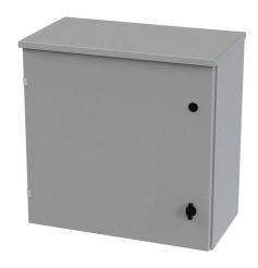
Saginaw enclosure, NEMA 3R, 24 x 24 x 12in (HxWxD), wall mount, carbon steel, ANSI 61 gray, powder coat finish, single-door, 1/4-turn padlocking wing handle.
