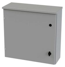
Saginaw enclosure, NEMA 3R, 24 x 24 x 8in (HxWxD), wall mount, carbon steel, ANSI 61 gray, powder coat finish, single-door, 1/4-turn padlocking wing handle.
