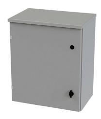
Saginaw enclosure, NEMA 3R, 24 x 20 x 12in (HxWxD), wall mount, carbon steel, ANSI 61 gray, powder coat finish, single-door, 1/4-turn padlocking wing handle.
