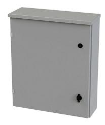
Saginaw enclosure, NEMA 3R, 24 x 20 x 6in (HxWxD), wall mount, carbon steel, ANSI 61 gray, powder coat finish, single-door, 1/4-turn padlocking wing handle.
