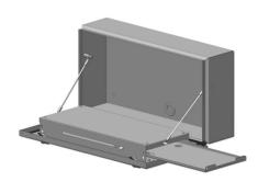
Saginaw keyboard housing, 12.25 x 24 x 6in (HxWxD), carbon steel, ANSI 61 gray. Mounting hardware included. Enviroline-type construction with ELJ hinge and mini 1/4-turn lever knobs.
