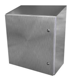
Saginaw sanitary enclosure, slope top, NEMA 3R/4/4X/12,  $24 \times 24 \times 12$ in (HxWxD), wall mount, 304 stainless steel, #4 brush finish, single-door, 1/4-turn sanitary stainless steel latch.
