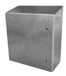
Saginaw sanitary enclosure, slope top, NEMA 3R/4/4X/12,  $24 \times 24 \times 10$  in (HxWxD), wall mount, 304 stainless steel, #4 brush finish, single-door, 1/4-turn sanitary stainless steel latch.
