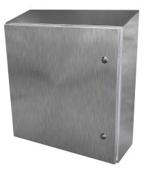
Saginaw sanitary enclosure, slope top, NEMA 3R/4/4X/12, 24 x 24 x 8in (HxWxD), wall mount, 304 stainless steel, #4 brush finish, single-door, 1/4-turn sanitary stainless steel latch.
