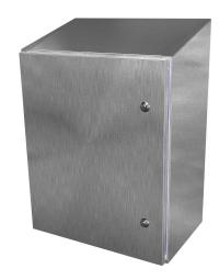
Saginaw sanitary enclosure, slope top, NEMA 3R/4/4X/12,  $24 \times 20 \times 12$ in (HxWxD), wall mount, 304 stainless steel, #4 brush finish, single-door, 1/4-turn sanitary stainless steel latch.
