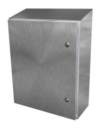
Saginaw sanitary enclosure, slope top, NEMA 3R/4/4X/12,  $24 \times 20 \times 8$ in (HxWxD), wall mount, 304 stainless steel, #4 brush finish, single-door, 1/4-turn sanitary stainless steel latch.
