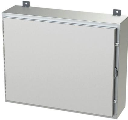
Saginaw enclosure, NEMA 3R/4/4X/12/13, 24 x 30 x 8in (HxWxD), wall mount, 304 stainless steel, #4 brush finish, single-door, stainless steel clamps, padlock hasp and staple.
