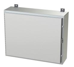
Saginaw enclosure, NEMA 3R/4/4X/12/13, 24 x 30 x 8in (HxWxD), wall mount, 316L stainless steel, #4 brush finish, single-door, stainless steel clamps, padlock hasp and staple.
