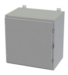
Saginaw enclosure, NEMA 3R/4/12/13, 24 x 24 x 16in (HxWxD), wall mount, carbon steel, ANSI 61 gray, powder coat finish, single-door, plated steel clamps, padlock hasp and staple.
