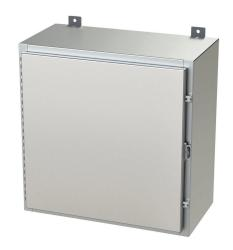
Saginaw enclosure, NEMA 3R/4/4X/12/13, 24 x 24 x 12in (HxWxD), wall mount, 316L stainless steel, #4 brush finish, single-door, stainless steel clamps, padlock hasp and staple.
