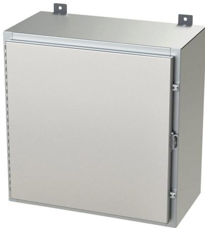
Saginaw enclosure, NEMA 3R/4/4X/12/13, 24 x 24 x 12in (HxWxD), wall mount, 316L stainless steel, #4 brush finish, single-door, stainless steel clamps, padlock hasp and staple.
