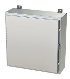
Saginaw enclosure, NEMA 3R/4/4X/12/13, 24 x 24 x 8in (HxWxD), wall mount, 304 stainless steel, #4 brush finish, single-door, stainless steel clamps, padlock hasp and staple.
