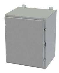
Saginaw enclosure, NEMA 3R/4/12/13, 24 x 20 x 16in (HxWxD), wall mount, carbon steel, ANSI 61 gray, powder coat finish, single-door, plated steel clamps, padlock hasp and staple.
