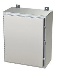
Saginaw enclosure, NEMA 3R/4/4X/12/13, 24 x 20 x 10in (HxWxD), wall mount, 316L stainless steel, #4 brush finish, single-door, stainless steel clamps, padlock hasp and staple.
