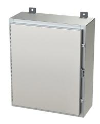
Saginaw enclosure, NEMA 3R/4/4X/12/13, 24 x 20 x 8in (HxWxD), wall mount, 304 stainless steel, #4 brush finish, single-door, stainless steel clamps, padlock hasp and staple.
