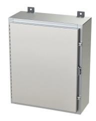
Saginaw enclosure, NEMA 3R/4/4X/12/13, 24 x 20 x 8in (HxWxD), wall mount, 316L stainless steel, #4 brush finish, single-door, stainless steel clamps, padlock hasp and staple.
