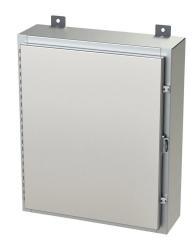
Saginaw enclosure, NEMA 3R/4/4X/12/13, 24 x 20 x 6in (HxWxD), wall mount, 304 stainless steel, #4 brush finish, single-door, stainless steel clamps, padlock hasp and staple.
