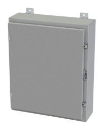
Saginaw enclosure, NEMA 3R/4/12/13, 24 x 20 x 6in (HxWxD), wall mount, carbon steel, ANSI 61 gray, powder coat finish, single-door, plated steel clamps, padlock hasp and staple.
