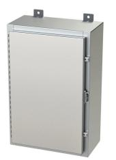
Saginaw enclosure, NEMA 3R/4/4X/12/13, 24 x 16 x 8in (HxWxD), wall mount, 304 stainless steel, #4 brush finish, single-door, stainless steel clamps, padlock hasp and staple.
