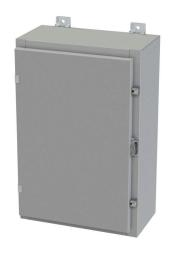
Saginaw enclosure, NEMA 3R/4/12/13, 24 x 16 x 8in (HxWxD), wall mount, carbon steel, ANSI 61 gray, powder coat finish, single-door, plated steel clamps, padlock hasp and staple.
