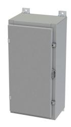
Saginaw enclosure, NEMA 3R/4/12/13, 24 x 12 x 8in (HxWxD), wall mount, carbon steel, ANSI 61 gray, powder coat finish, single-door, plated steel clamps, padlock hasp and staple.
