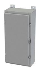
Saginaw enclosure, NEMA 3R/4/12/13, 24 x 12 x 6in (HxWxD), wall mount, carbon steel, ANSI 61 gray, powder coat finish, single-door, plated steel clamps, padlock hasp and staple.
