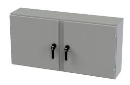
Saginaw Enviroline series enclosure, NEMA 3R/4/12/13, 24 x 48 x 10in (HxWxD), wall mount, carbon steel, ANSI 61 gray, powder coat finish, 2-door, 3-point keylocking/padlocking combo handle.
