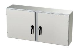
Saginaw Enviroline series enclosure, NEMA 3R/4/4X/12/13, 24 x 48 x 10in (HxWxD), wall mount, 304 stainless steel, #4 brush finish, 2-door, 3-point keylocking/padlocking combo handle.
