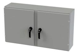
Saginaw Enviroline series enclosure, NEMA 3R/4/12/13, 24 x 42 x 10in (HxWxD), wall mount, carbon steel, ANSI 61 gray, powder coat finish, 2-door, 3-point keylocking/padlocking combo handle.
